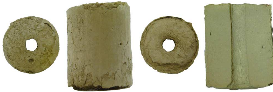
Fig. 4. Sintered annular ZrN pellet fabricated by DCC (outer diameter: 9.7 mm) and cut for ceramography on right side.
