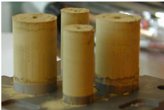
Fig. 5. Green annular ZrN pellets fabricated by FD (outer diameters: 10–15 mm) before thermal drying step.
